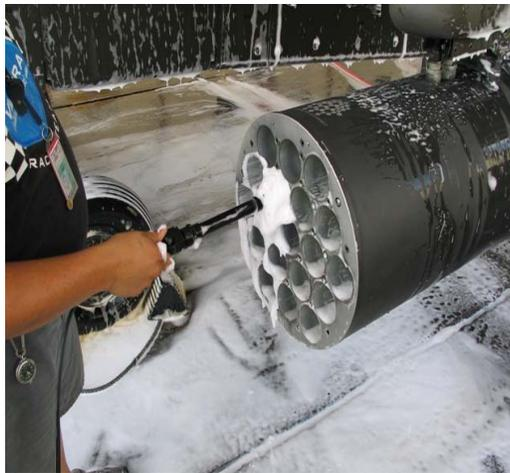
*Foaming brush applicator that is applying 725 Cleaner/Degreaser to a rocket pod.*
